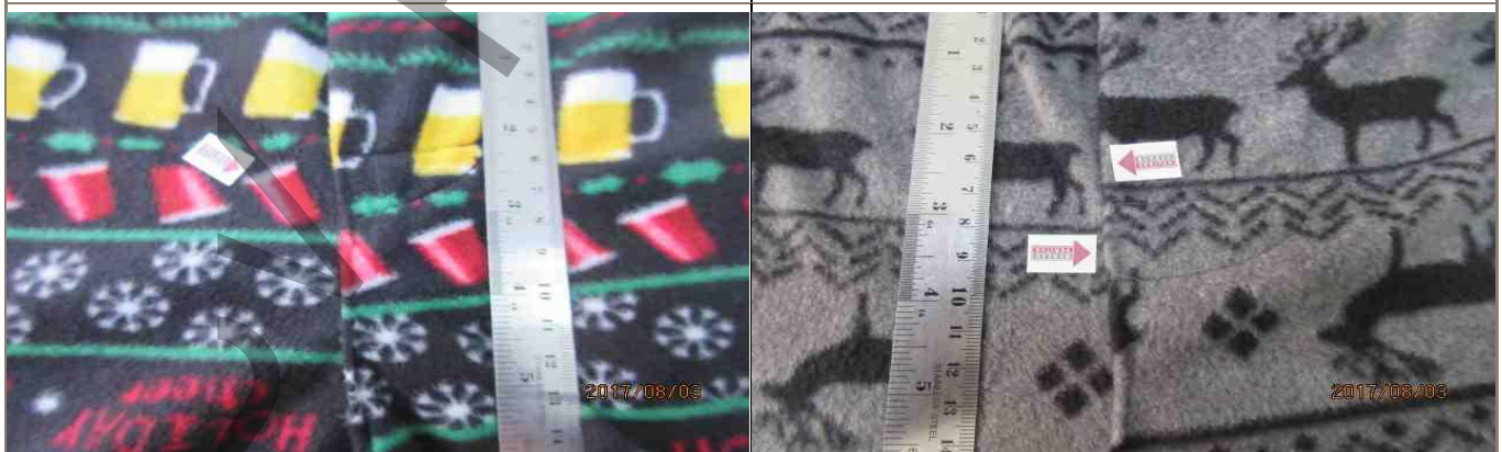
Obvious misaligned stripes
