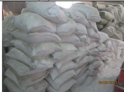
(17) MGO materials not identified in raw materials warehouse
